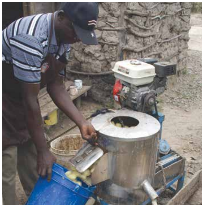
To reduce labour through manual Njoroge uses a potato peeling machine
