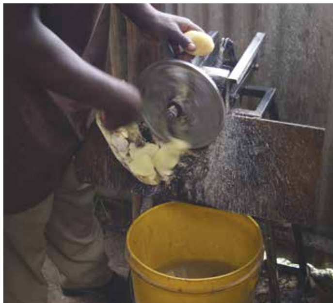
A fabricated machine is used for chopping the potatoes
