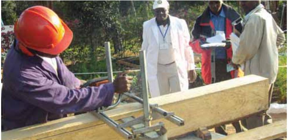
production. To produce uniform size timber all split saws should be fitted with chain saw frame (see picture), the chain saw frame helps guide the split saws along the cutting path to produce quality timber that is uniform in size from one end to the other. Lumberjacks using the chain saw frame have managed to recover up to 57 per cent of timber that would have been wasted during production.
