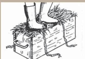
**Step 1:** The box is filled with hay and tightly compacted.
