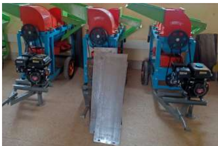
Figure 1: Motorized legume threshers with multiple sieves
