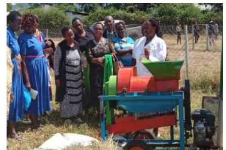
Fig 2: Testing of motorized legume thresher
