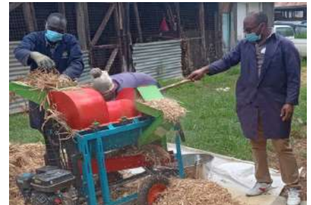
Fig 2: Testing of motorized legume thresher
