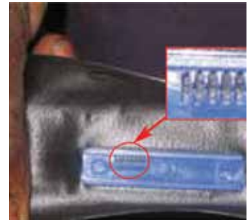
Checking emitters for blockage
